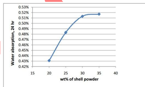
Fig2.7: Water absorption of coconut particle reinforced composite in 24 hr
